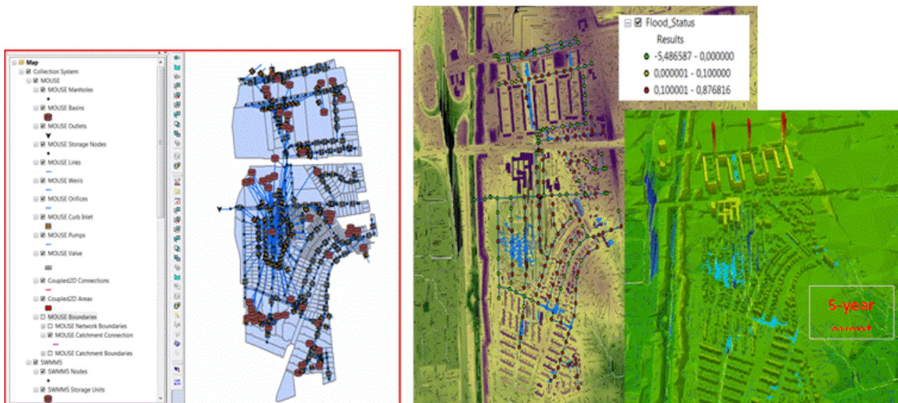
Figure 4: Flood model where Basins, weirs, orifices and flow accumulation paths formulate the 1D model on the surface is connected to the 1-D model beneath surface of pipe net, rivers and channels (Left). A 5-year event flood map in Horsedammen compared to node flood map (Middle). And a 3D dynamic flood map of a 5-year event (Right).
