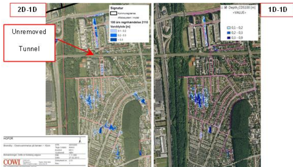
Figure 8: Comparison between a CDS100 in the traditional flood modelling (Left) and in the method suggested in this paper (Right).
