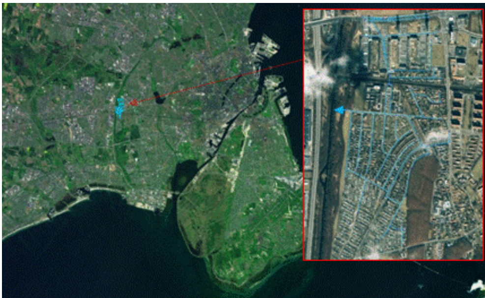
Figure 1: Location of Horsedammen due to Copenhagen. The blue lines are the rainwater pipe net of this study.
