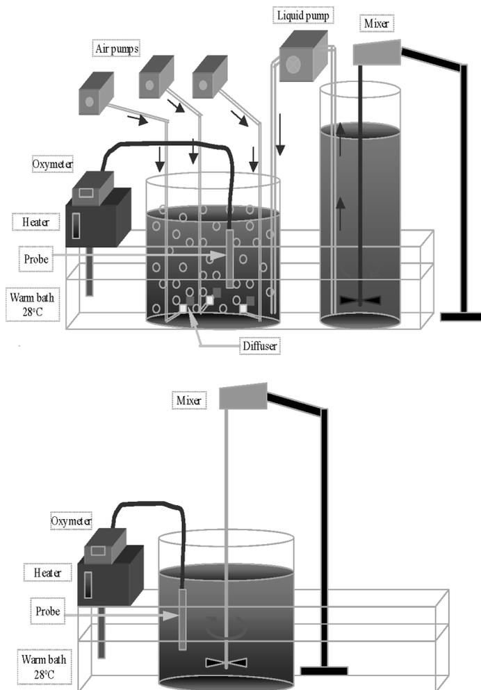
**Figure 1** Schematic illustration for the experimental rig: During slow aerated fill and aeration. The wastewater was pumped from a tank into the reactor (Top). The experiment during mixing with no aeration (Bottom)
