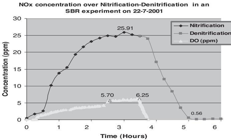
**Figure 2** NO<sub>x</sub><sup>-</sup> and dissolved oxygen (DO) concentrations during nitrification–denitrification in SBR
