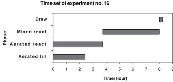
**Figure 4** Selected cycle time for the modelling (exp. no. 16)
