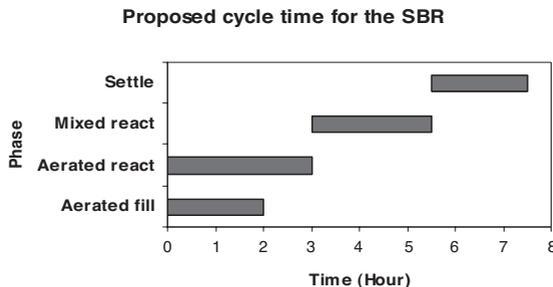
**Figure 3** Proposed cycle time for the SBR experiment
