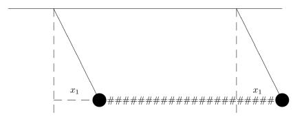
The two pendulums swing together in phase and of course, since the two pendulums are identical, the spring is neither stretched nor compressed. Effectively the spring doesn't influence this mode at all. It is therefore not surprising that the frequency  $\omega_1 = \sqrt{g/\ell}$  is just the same as that for a free pendulum of the same length. In normal mode 1, we have  $y_1 = 0$ , and so  $x_1 = -x_2 = y_2/\sqrt{2}$ .
