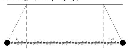
The two pendulums oscillate out of phase, with the spring being alternately stretched and compressed. Compared to the first normal mode, the restoring forces are here <u>increased</u> because the spring is contributing something. Hence the frequency is higher:
