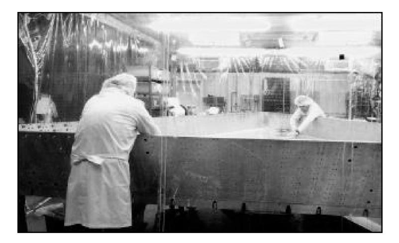
A **calorimeter** is a device that helps scientists measure the energy of a particle. This triangular section is layered with sheets of **lead and plastic**. The lead is heavy and dense, so the particles have a hard time going through it. Scientists can tell how much energy a particle had by seeing how much lead it took to stop it.
