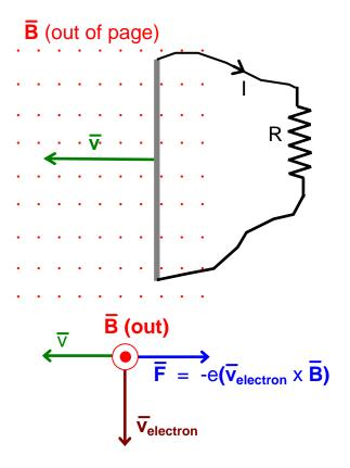
The overall force on the wire is  $F_{mag} = \Sigma F$  for all the electrons.
