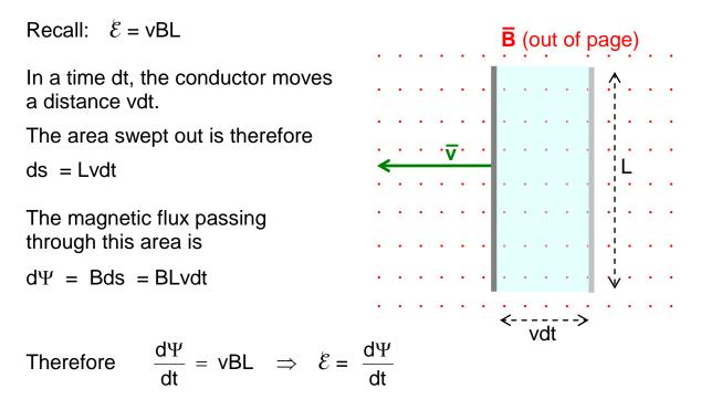
The induced emf is equal to the rate of sweeping out of magnetic flux
