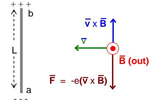
Induced emf  $\mathcal{E}$  = work done to move a unit positive charge from a to b against the magnetic force
