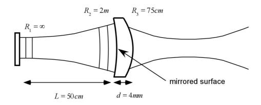
Find the spot-size of the laser beam at the plane mirror [4]
