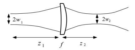
By finding the ray transfer matrix describing the propagation of the beam between the waists and applying the ABCD law, determine  $w_2$  and  $z_2$ .
