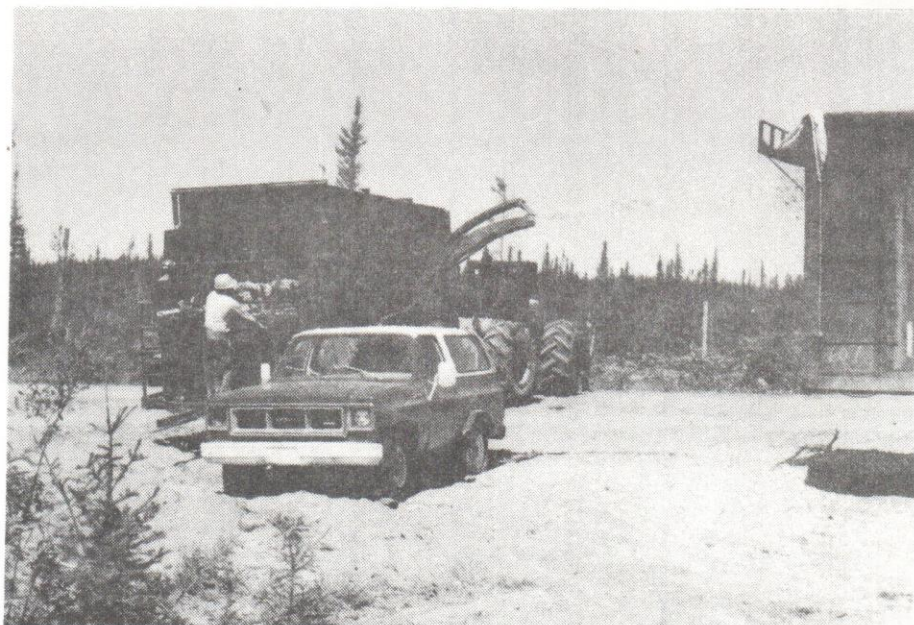
Figure 28. Operation of Transfer Blower: Chips Moving from Chip Wagon to Highway Van
