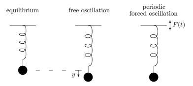
The force exerted by the spring is a negative multiple of y: we will choose k so that the force is  $-mk^2y$ . Unforced system The governing equation is
