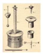
Figure 2: Coulomb's torsion balance
