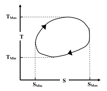
we can express the area under a curve in the T - S plane as (I take T on the vertical axis and S on the horizontal axis)
