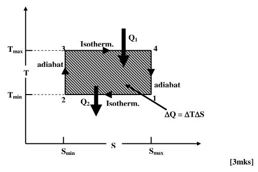
(d) To compare the general engine shown in (b) with the Carnot engine shown in (c), enclose the general cycle in the smallest rectangle that will just hold it, i.e., a rectangle with horizontal sides at  $T_{\text{max}}$  and  $T_{\text{min}}$  and with vertical sides at  $S_{\text{max}}$  and  $S_{\text{min}}$
