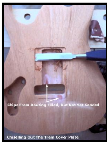
Figure 4 – The tremolo cavity being routed. See footnote 3
