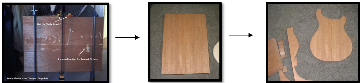
Figure 2.2 – See footnote 4 An outline of the body is traced onto the body blank.
