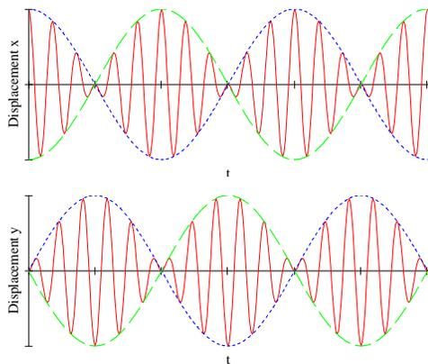
Figure T7.4: Interchange of energy between two coupled pendulums.
