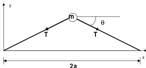
Figure T7.1: A single bead on a stretched wire acting as a simple harmonic oscillator.
