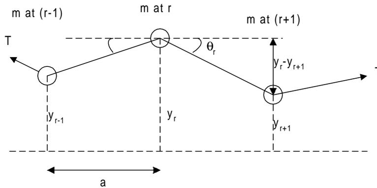
Figure T7.2: Displacements on a regularly beaded string.
