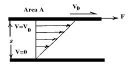
Figure 2.5-2. Viscosity experiment.
