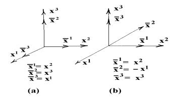
Figure 2.5-1. Coordinate transformations due to rotations
