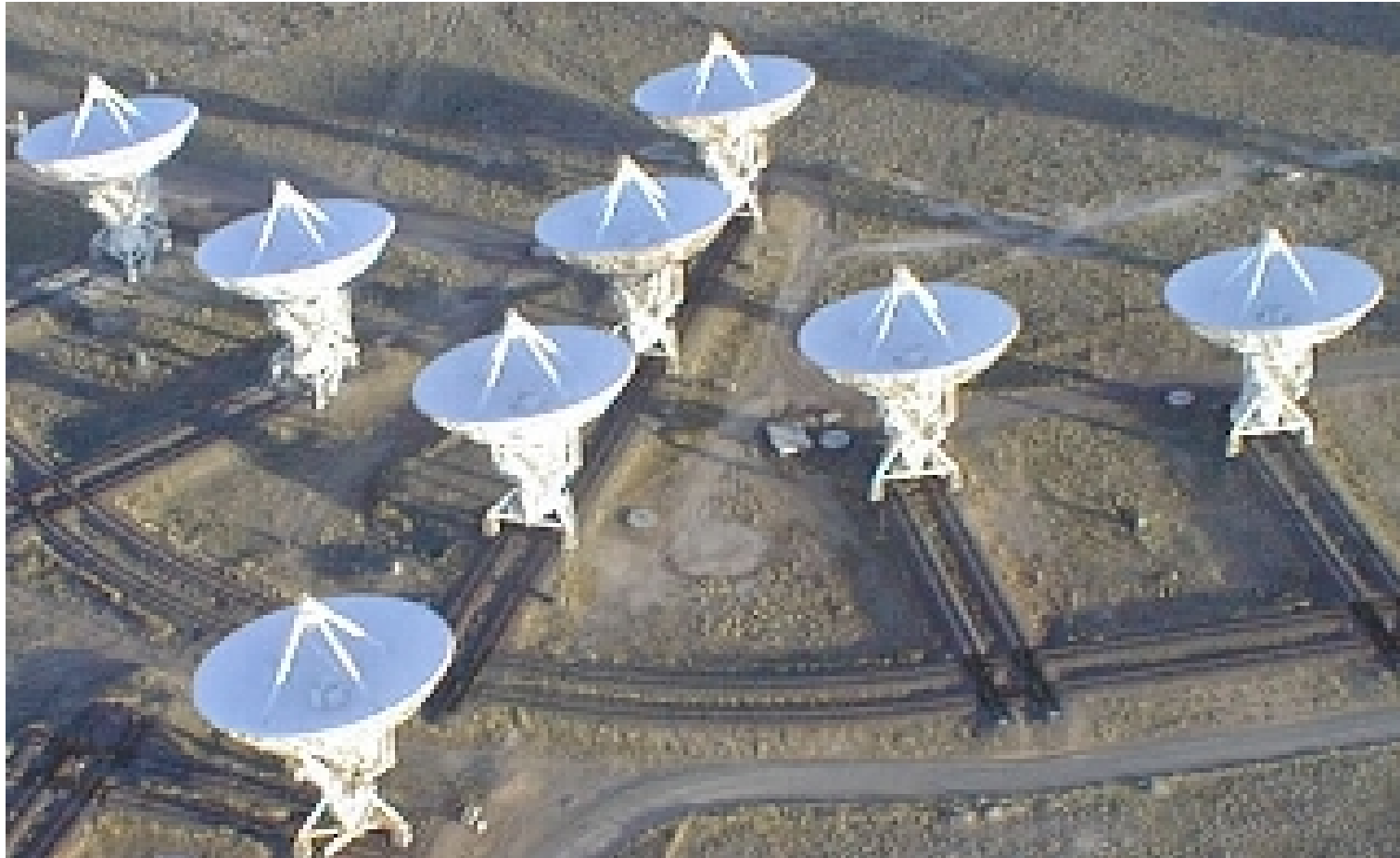
Very Large Array in New Mexico. Radio interferometer, 73 MHz—43 GHz. 27 antennae, baselines up to 36 km.
