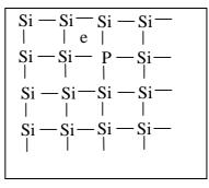
weakly bound to the phosphorus and at room temperatures it is easily excited into the conduction band. This impurity has *donated* an electron from a *donor state*. The
