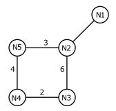
The net work uses a Distance Vector Routing protocol. Once the routes have stabilized, the distance vectors at different nodes are as following
