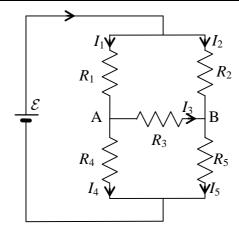
What is the effective resistance of the network above? When connected to a source of EMF as shown, what are the potentials at points A & B (with respect to the negative side of the battery)?
