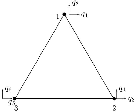
**Fig. 5:** Coordinates for the 3 particle-spring system.
