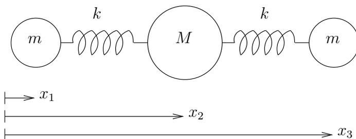
**Fig. 4:** A simple model of a CO<sub>2</sub> molecule.
