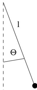
**Fig. 1:** A simple pendulum of length  $l$  with a mass  $m$ .
