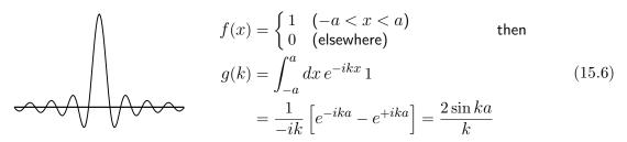
The first observation is of course that the dimensions check: If dx is a length then so is 1/k. After that, there is only one parameter that you can vary, and that's a. As a increases, obviously the width of the function f increases, but now look at g. The first place where g(k)=0 is at  $ka=\pi$ . This value,  $\pi/a$  decreases as a increases. As f gets broader, g gets narrower (and taller). This is a general property of these Fourier transform pairs.
