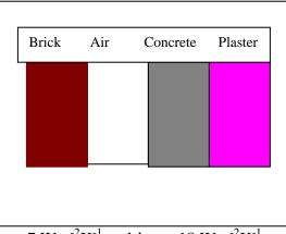
coefficients. Typical values for these would be  $h_{in} = 7 \text{ Wm}^{-2}\text{K}^{-1}$  and  $h_{out} = 18 \text{ Wm}^{-2}\text{K}^{-1}$ . This gives a final *U-value* of 0.56Wm<sup>-2</sup>K<sup>-1</sup>
