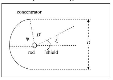
entering the trough per unit length is also *D*. The irradiance from the sun is *I*. The rod will lose energy by radiation. Radiation that goes towards the trough is lost since it goes
