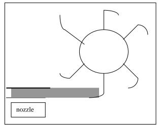
respect to the frame of reference of the cup, the speed of the water jet is  $(u_j - u_t)$  both before and after the water hits the cup. (The direction of course is reversed). This is also the *change* of velocity seen in the laboratory frame. Thus the change of momentum of the fluid (and thus the force exerted on the cup) is
