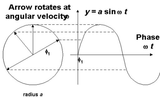
The relationship between a phasor diagram and sinusoidal variation
