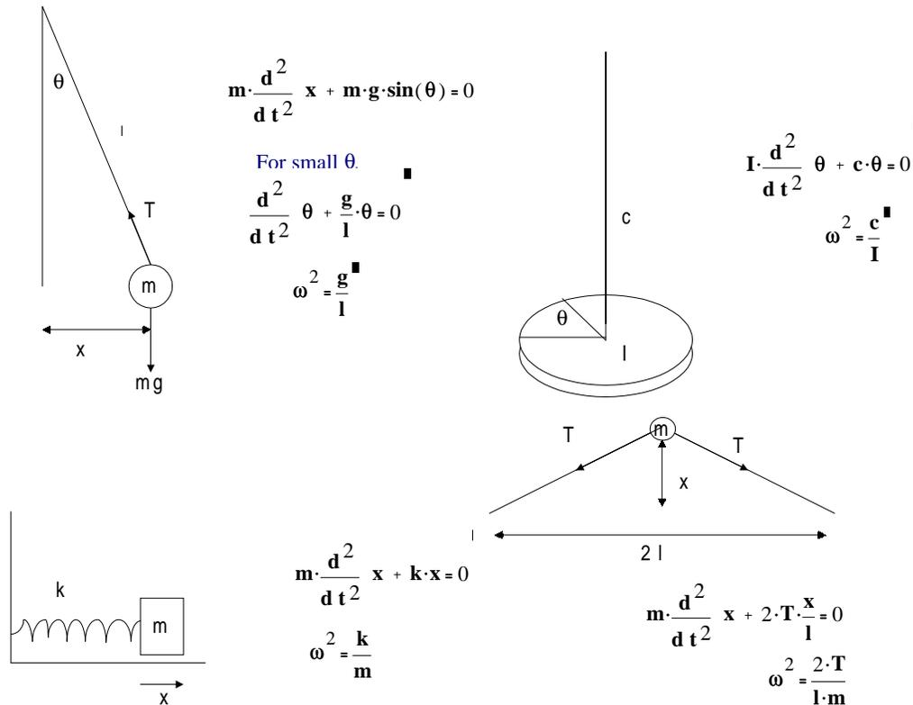
Figure 0.1: A selection of simple harmonic oscillators.
