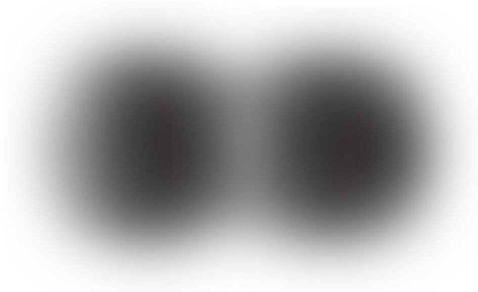
Figure 11: Negative charge density ( \propto |\psi|^2 ) produced by the electron in the \text{H}_2^+ molecular ion.
