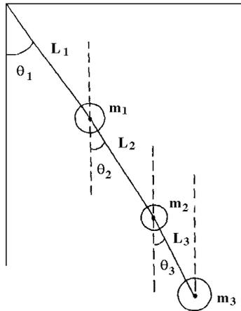
Figure 2.2-8. Compound pendulum
