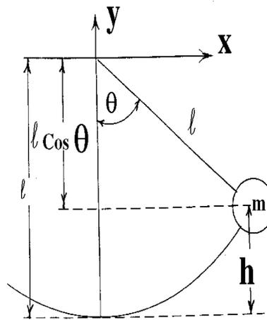
Figure 2.2-3 Simple pendulum system
