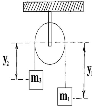
Figure 2.2-2 Simply pulley system
