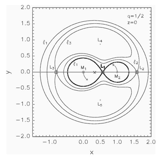
Critical equipotential which passes through the inner Lagrangian point  $L_1$  defines the Roche lobes of the two stars.  $L_1$  is a *saddle point* of the potential – ie gas bound to one star in the vicinity of  $L_1$ finds it easier to pass through  $L_1$  onto the other star than to escape completely.
