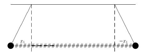
The two pendulums oscillate out of phase: the spring is alternately stretched and compressed. Compared to the first normal mode, the restoring forces are here <u>increased</u> because the spring is contributing something. Hence the frequency is higher:
