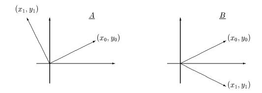
For the combination  $\underline{B}\underline{A}$ , we first act with  $\underline{A}$  and then  $\underline{B}$ . In the case of  $\underline{A}\underline{B}$  it is the other way around and this leads to a different result, as shown in the picture.
