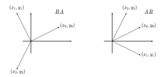
Clearly the end point  $(x_2, y_2)$  is different in the two cases so that the operations corresponding to  $\underline{A}$  and  $\underline{B}$  obviously don't commute. We now want to show exactly the same results using matrix manipulation, in order to illustrate the power of matrix multiplication.
