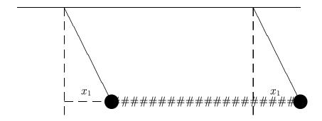
The two pendulums swing together in phase and of course, since the two pendulums are identical, the spring is neither stretched nor compressed. Effectively the spring doesn't influence this mode at all. Frequency  $\omega_1 = \sqrt{g/\ell}$  is that for a free pendulum of the same length.
