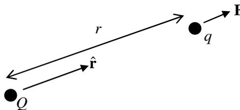
Figure 2 The force on  $q$  due to  $Q$
