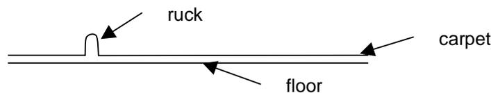
The motion produces slip between the upper and lower parts of the crystal. The direction and magnitude of this slip is given by the Burgers vector  $\vec{b}$ . This characterises a dislocation. For an edge dislocation, the slip is perpendicular to the direction, or 'sense' of the dislocation line. This is a vector which is tangent to the dislocation line.  $b$ , the magnitude of  $\vec{b}$ , is often equal to a lattice spacing.
