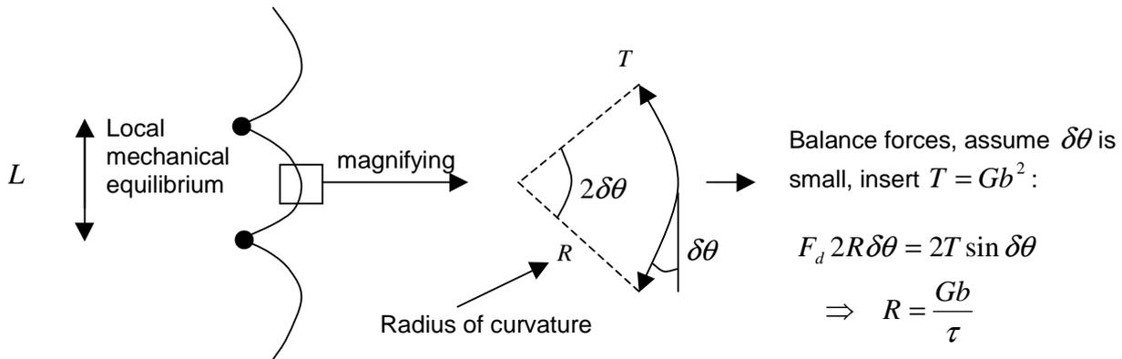
As the stress increases, the bowing radius decreases. But  $R$  can not be less than  $L/2$  where  $L$  is the separation of pinning centres. Yield occurs at  $R = L/2$ , i.e. for a semicircular bowed dislocation line. Dislocation is unpinned: escape corresponds to yield.
