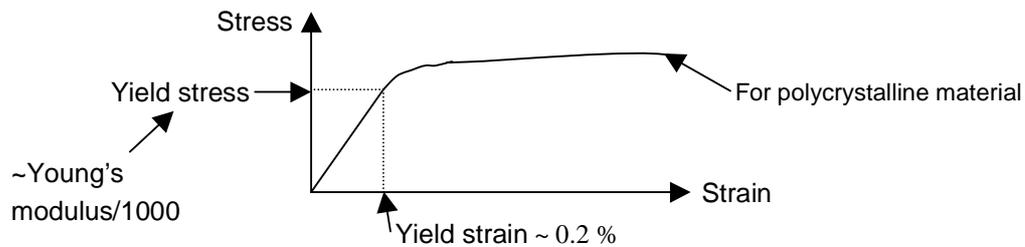
Plastic strains (those which do not vanish when the stress is removed) occur due to shear stresses, even when the applied stress is tensile. Slip occurs along 'slip planes' when the yield stress is exceeded.
