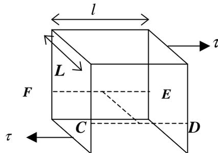
If a dislocation on the slip plane  $CDEF$  moves from  $CF$  to  $DE$ , the upper block slips a distance  $b$  to the right. Work done is shear force times distance moved, i.e.  $\tau A b$  with  $A = Ll$ .
