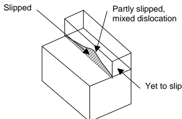
Glide of dislocations is brought about by relatively low shear stress, only small distortions and rearrangement of atoms are needed.
