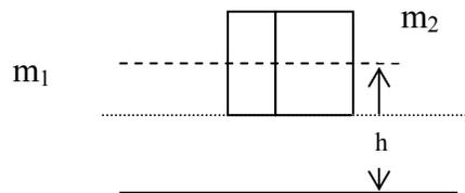
a-2) Iron object shifted far away from the magnet. Using an **external force  $F_{\text{ext}}$** , one detaches  $m_1$  from magnet and shifts it far away (no magnetic interaction  $m_1$ - $m_2$ ).
