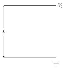
What is the potential between the two plates? You all know that the answer must be  $V = V_0 z/L$  but we are going to derive this by solving the partial differential equation. This will demonstrate the techniques to be used in more complex cases.
